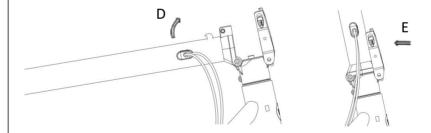
WARNING: Be sure to fold down the stem hook when the scooter is unfolded and ready for use.
